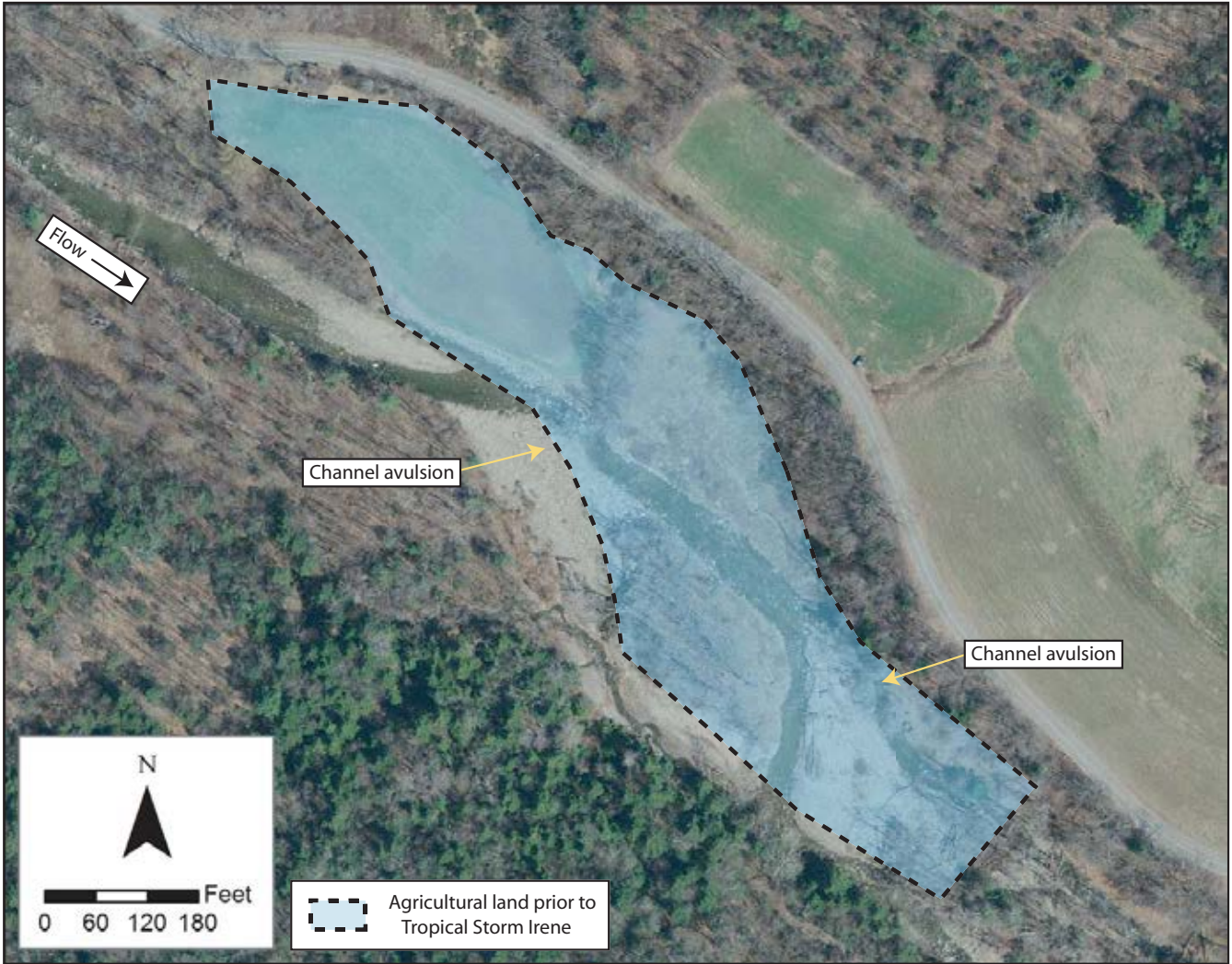
Conservation of attenuation assets and encroachment removal - West Branch North River. 2014 aerial photo showing flood-damaged riparian lands and extent of agricultural use prior to Tropical Storm Irene.
